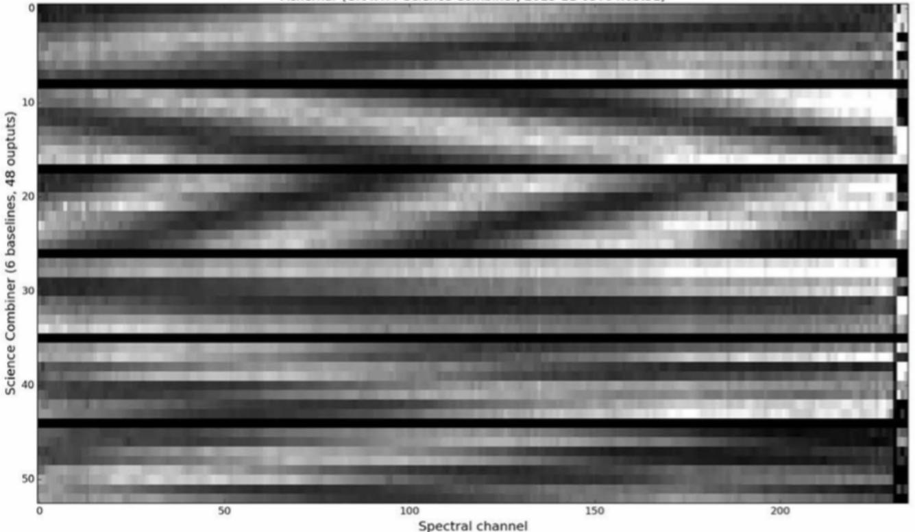
48 spectrally resolved channels: 2 (polarisation) x 4 (ABCD) x 6 baselines
