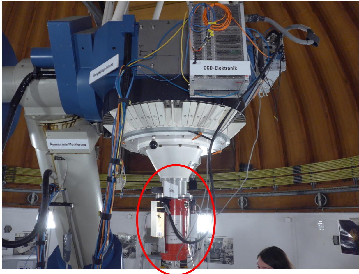
Figure 1-1: CCD's dewar installed at the Cassegrain focus of the telescope.
