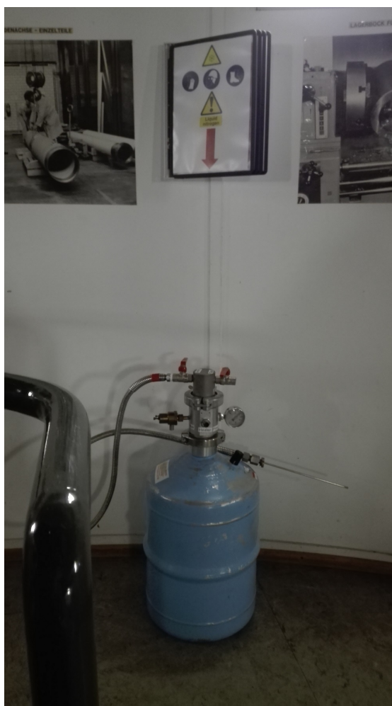
Figure 5: Liquid Nitrogen vessel kept at its designated position in the telescope room. Read and follow the safety instructions displayed in the black panes located above the vessel.
