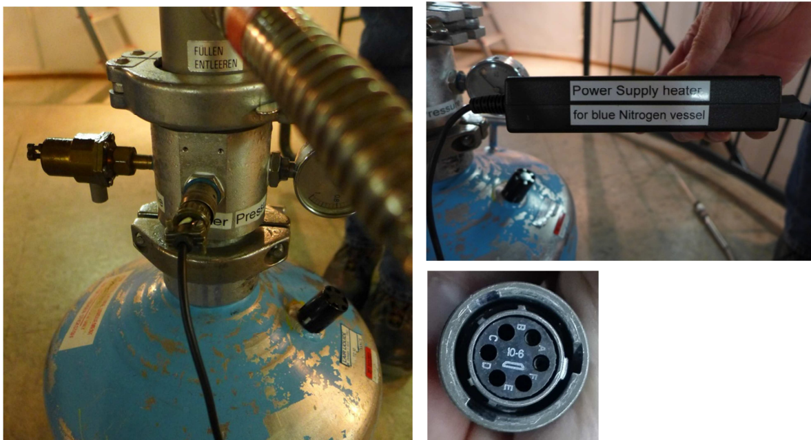
Figure 4-2: Left: vessel with heater connected. Right up: power supply for heater. Right down: heater connector.
