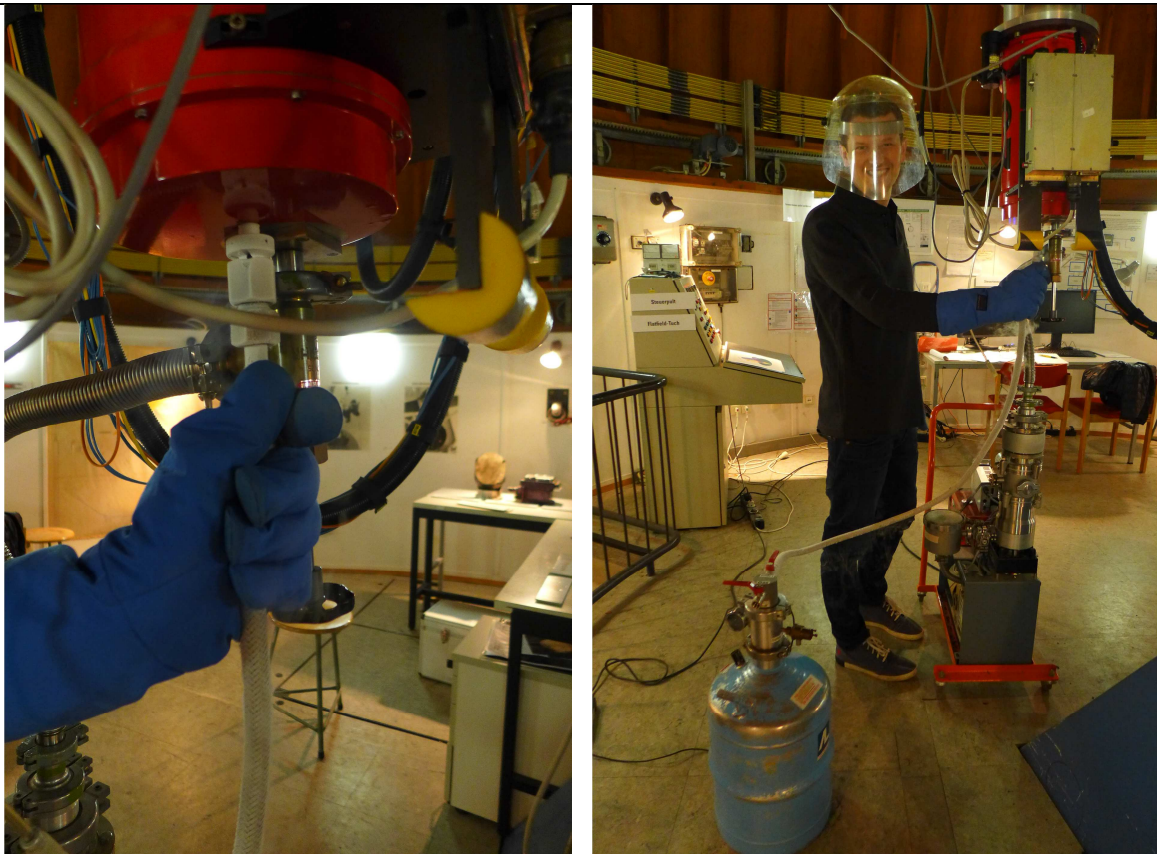
Figure 6-2: Filling LN 2 with face protection.
