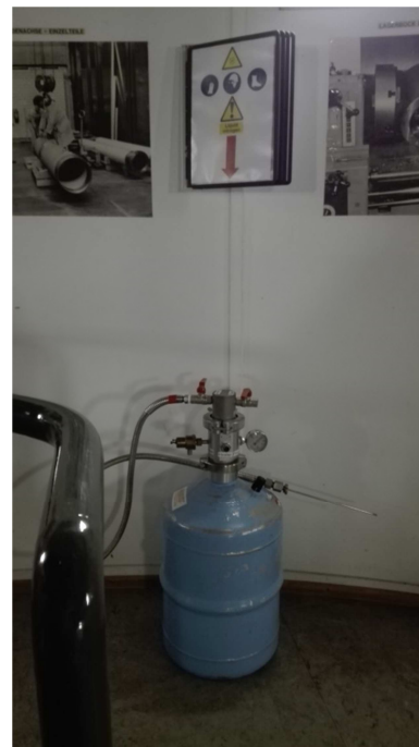
Figure 2-1: Left: location of the protection equipment. Right: Safety sheets location, on the wall above the small blue LN 2 vessel.
