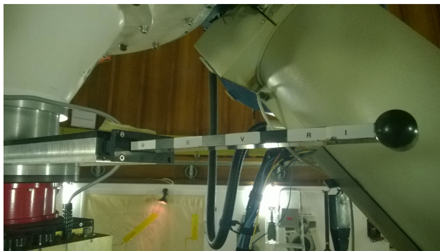
Figure 6-1: Aluminium box where the filters are installed: Opened.
