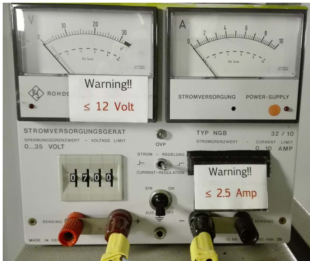
Figure 6-3: Power supply of the lamp use for the dome flat field.
