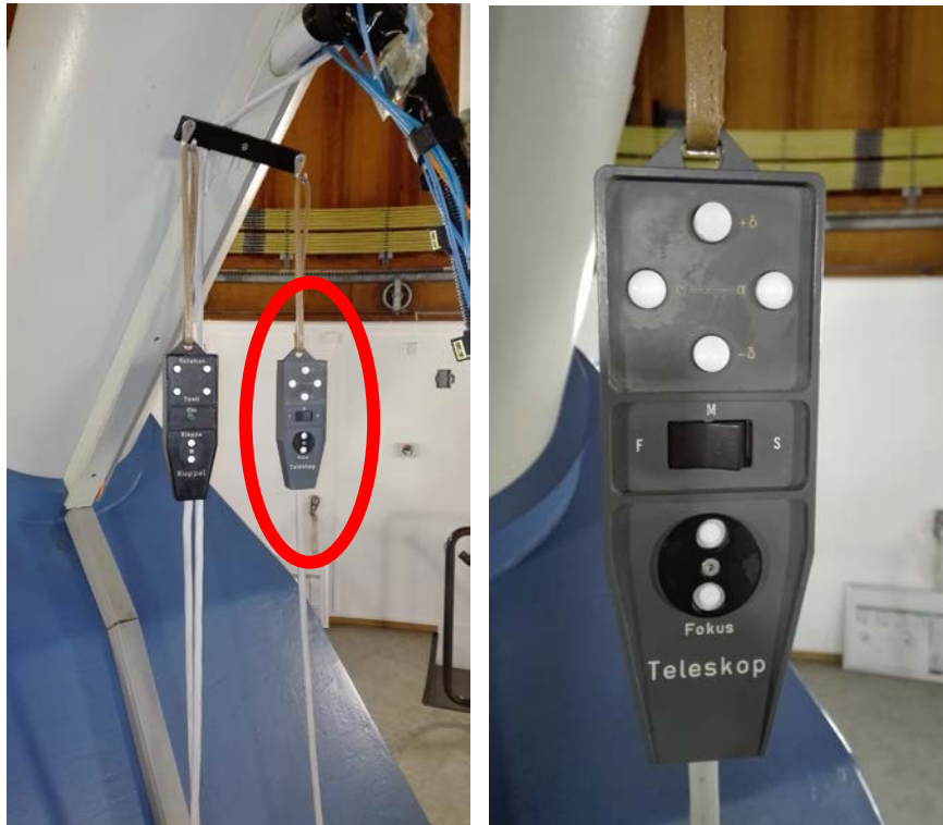
Figure 5-2: Left: position of the manual control for the telescope hanging at the telescope. Right: control itself.
