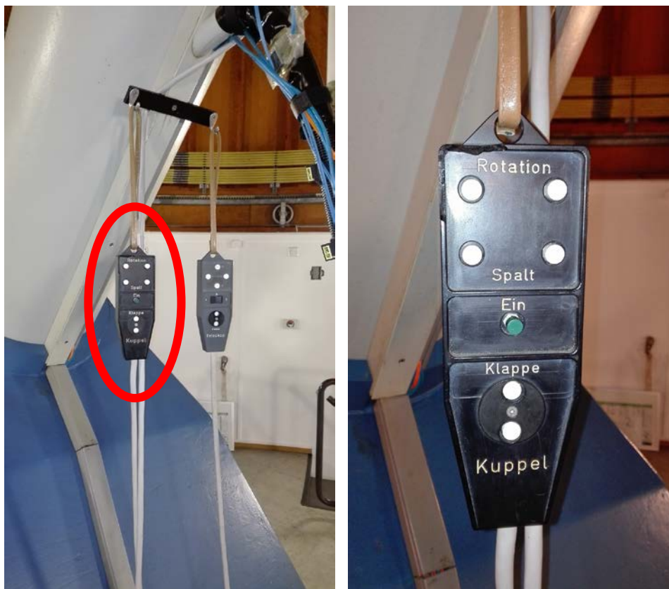
Figure 4-1: Left: position of the manual control for the telescope dome hanging at the telescope. Right: control itself.
